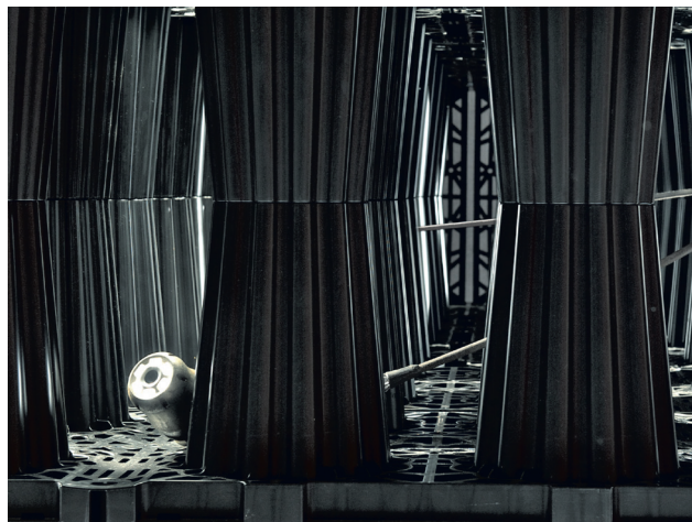
Camera checking the internal spaces
